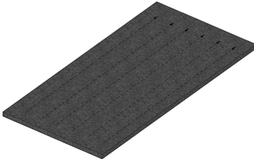
Figure 1 - Apply glue longitudinally
